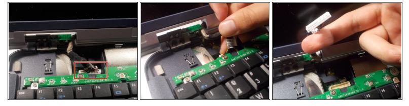
• Remove the connection from the exposed hinge and interior of the device
