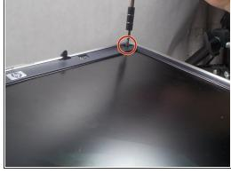
Unscrew the six 5.0 mm Philips #0 screws underneath the caps
