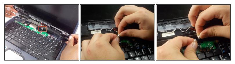
Remove the connection between the plastic case and interior of the device
