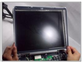
• Using a spudger, pry the plastic casing off of the screen.
