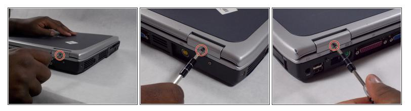
Remove two 5.0 mm Philips #0 screws on the hinge of the device
