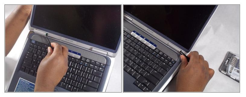
Using tweezers, gently pull on the hinges to remove the plastic case connected to the hinges
