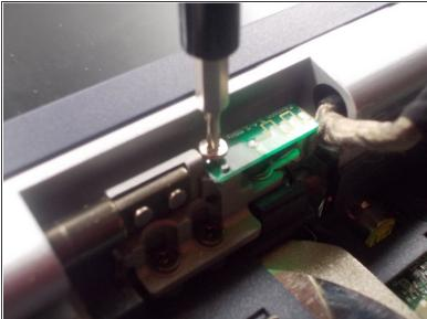
Remove the 3.5 mm philips #00 screw on the small circuit board on the hinge
