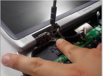
Remove the 5.0 mm philips #0 screw that was hidden underneath the small circuit board
