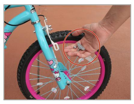
Remove the brake pads from the calipers.
