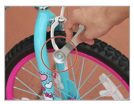
Reattach the brake pads to the calipers and tighten them with the 10mm wrench so that the leading edge of the brake sits closer to the rim than the rear edge.
