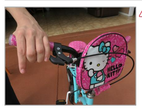
Test the brake to ensure that it functions properly before riding the bike.
