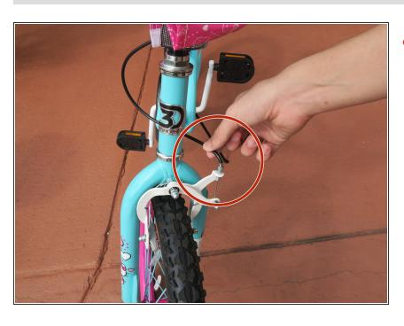
Check the brake cable and make sure that it is still connected and secured to the brake calipers.
