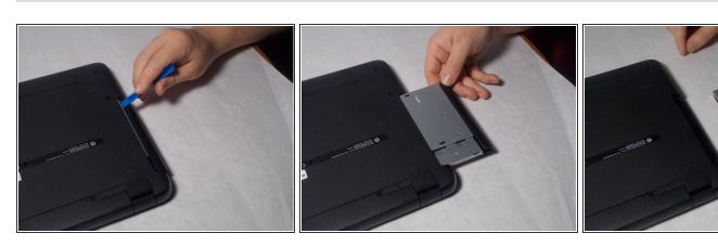
Remove the disk tray assembly by sliding it out from the side using the blue plastic opening tool.
