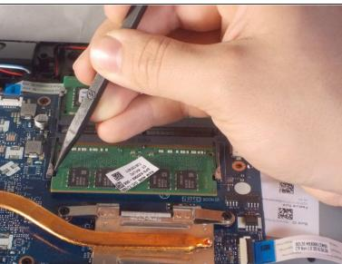
Using a plastic spudger, unclip the latch locking the RAM to the motherboard.
