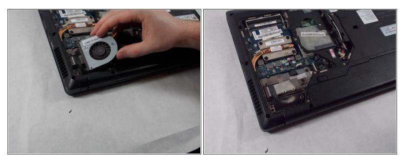
• Remove the fan by pulling it up and away from the computer.
