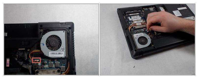
• Carefully pull the fan's power connector from the laptop.
