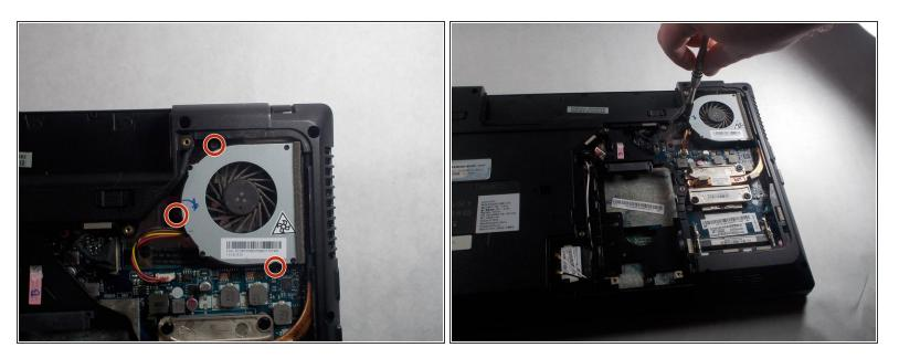
• Remove the three 5mm Phillips #1 screws holding the fan in place.
