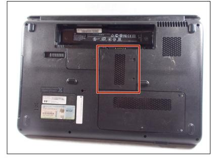
Locate RAM access door on the bottom side of the laptop.
