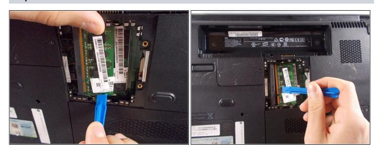
Gently pull apart the two metal tabs located on both sides of the stick of RAM.
