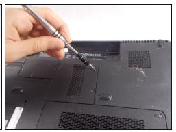
Remove the two screws holding down the RAM access door with a Phillips #1 screwdriver.
