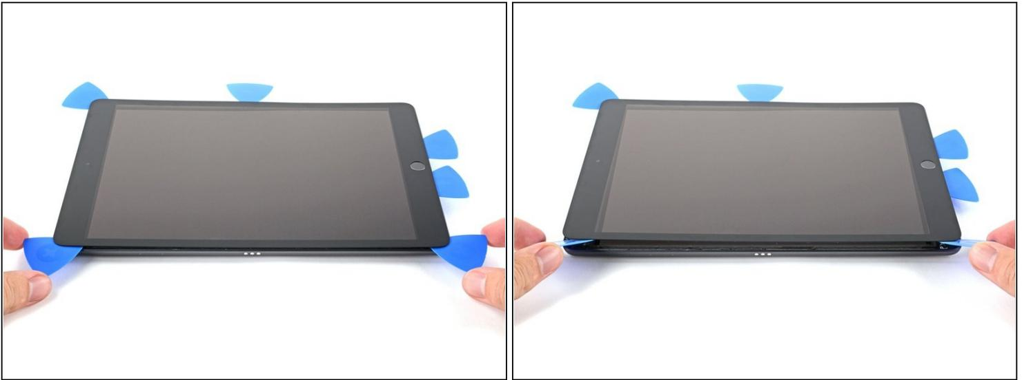
**⚠ Be very careful with this step.** Take your time, ensure the adhesive is hot and soft, and make sure you separated all of the adhesive with a pick. Don't be afraid to stop and reheat.
