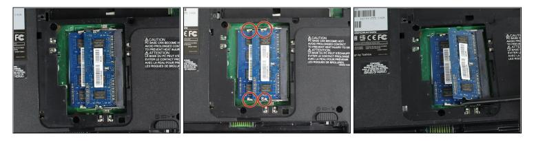
Take the nylon spudger, and push the prongs so that it releases the RAM.
