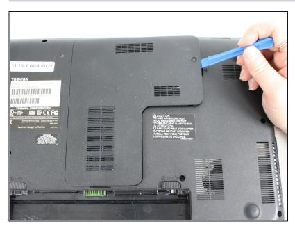
Use the plastic opening tool to pry the panel open. Be sure to do this on all four sides. Then the panel will lift off.
