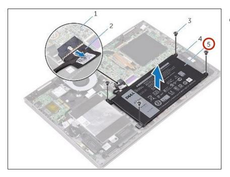
• Lift the battery off the palm-rest assembly.
