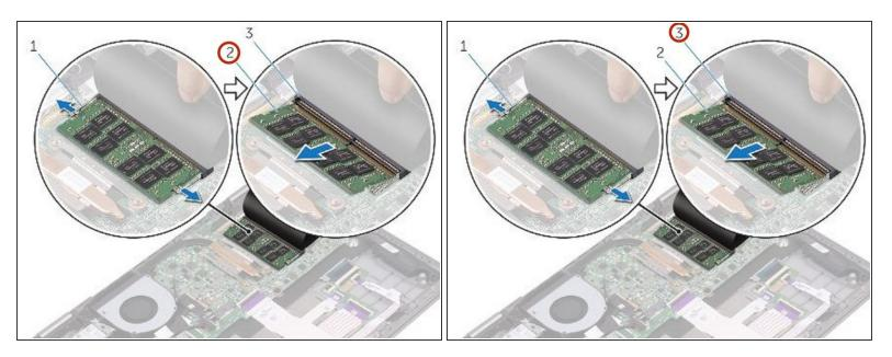
• Remove the memory module from the memory-module slot.
