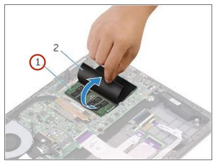
Use your fingertips to carefully spread apart the securing-clips on each end of the memory-module slot until the memory module pops up.
