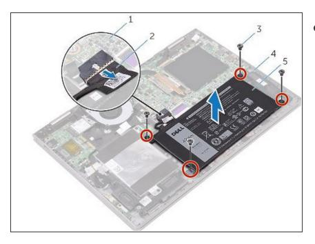
Align the screw holes on the battery with the screw holes on the palmrest assembly.
