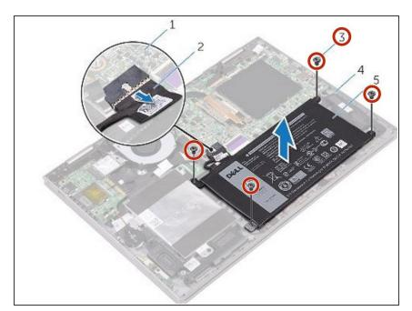
• Remove the screws that secure the battery to the palm-rest assembly.
