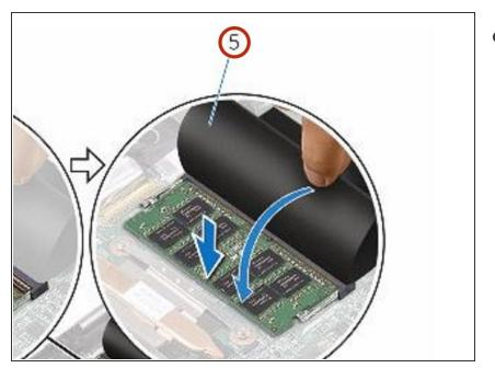
• Lift the Mylar to access the memorymodule slot.
