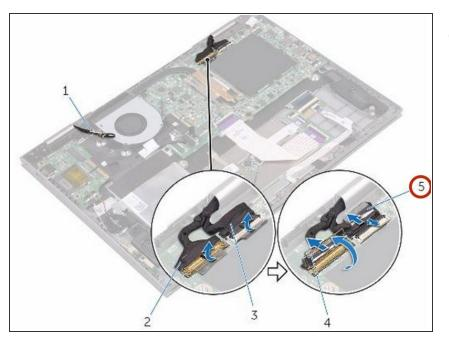
Adhere the pieces of tape that secure the display cable and the touch-screen board-cable to their respective connectors on the system board.
