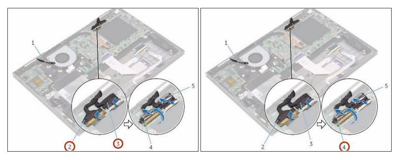
Slide the display cable and the touch-screen board-cable into their respective connectors on the system board and close the latches to secure the cables.
