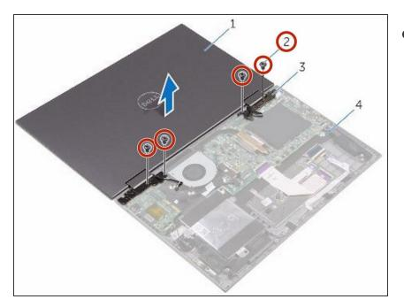
Remove the screws that secure the display assembly to the palm-rest assembly.
