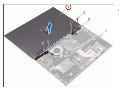
Place the NEW display assembly face down on the palm-rest assembly.
