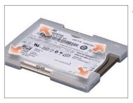
Remove the hard drive from the rubber case.
