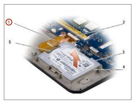
Attach the hard drive cable to the hard-drive system board connector.
