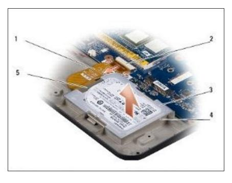
Place the **NEW** hard drive in the hard drive compartment.
