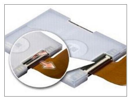
Detach the hard drive cable from the hard drive cable connector.
