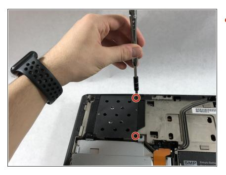
Unscrew the two 6.35 mm using the PH1 screw driver.
