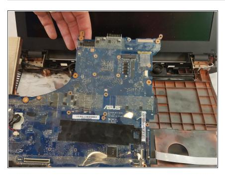
Ensuring no missed connections or screws, remove the motherboard from the assembly.
