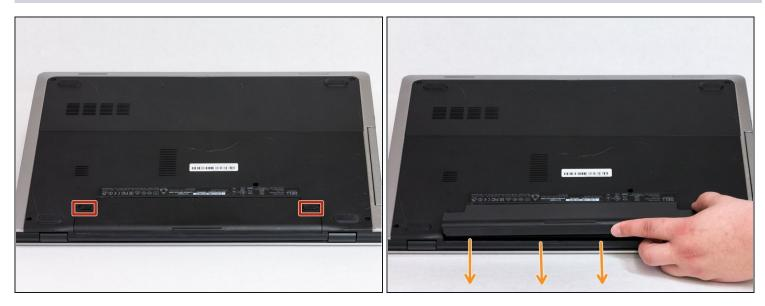
(i) First carefully turn the laptop over so you can access the battery.
