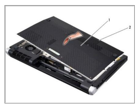
Loosen the ten captive screws on the base cover and lift the cover off the computer at an angle as shown in the figure.
