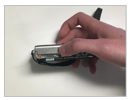
Slide the battery door open with a finger or thumb and release it so the door opens.
