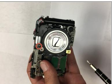
Remove the two 3mm Phillips #000 screws.
