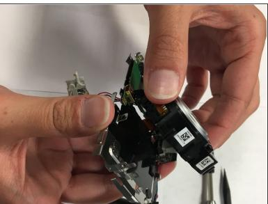
Use the flat end of a spudger to pry the lens locking tabs open while pulling the lens away from the camera body.
