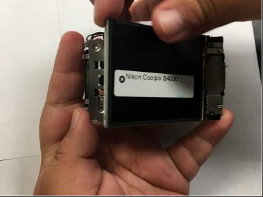
Grabbing the top left corner of the screen, pull it up until the screen comes completely off.
