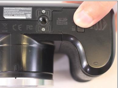
Slide switch to open lock position.
