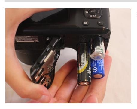
Remove the batteries.
