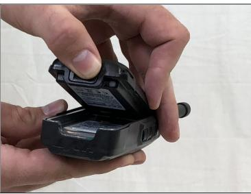
• Push in the release button and pull up on the battery to remove.
