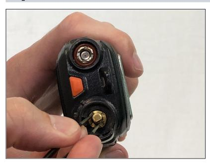
Remove the brass washer from the base of the antenna slot by turning it counterclockwise with a set of tweezers.
