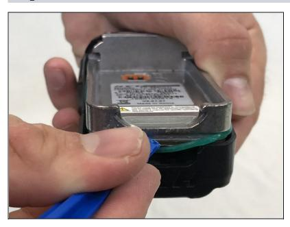
Using a plastic opening tool, pry in between the plastic case and metal circuit board to remove the board.
