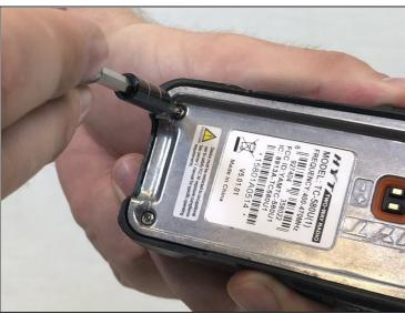
• Remove the two 15mm T8 Torx screws from the base of the battery cavity.
