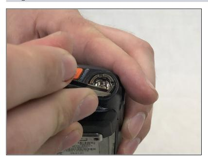
Remove grey nut from base of volume knob by turning it counterclockwise with a set of tweezers.
