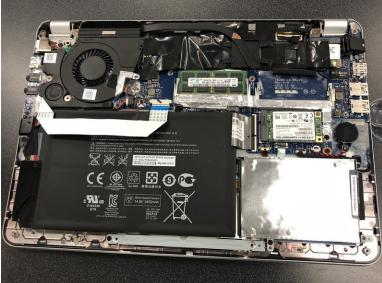
Pull the panel up and off to remove from the laptop.
