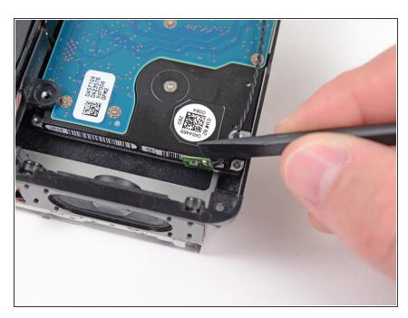
Use the flat end of a spudger to pry the hard drive thermal sensor board off the adhesive securing it to the side of the hard drive.
