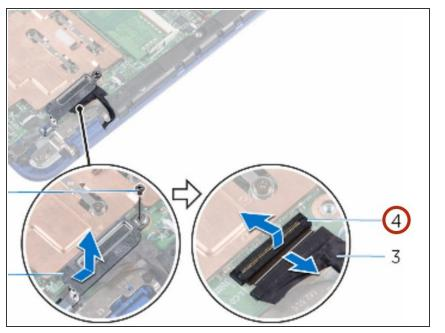
Slide the display-cable bracket into the slot on the palm rest and keyboard assembly.
