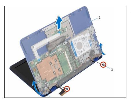
Replace the screws that secure the display assembly to the palm rest and keyboard assembly.
