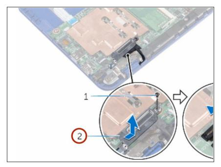
• Slide and lift the display-cable bracket off the system board.
