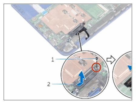
Align the screw hole on the displaycable bracket with the screw hole on the system board.
