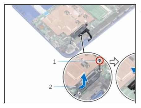
Replace the screw that secures the display-cable bracket to the system board.
