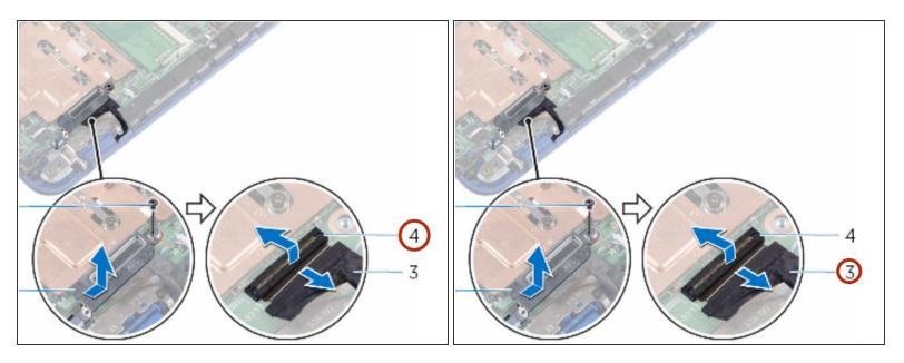
• Open the latch and disconnect the display cable from the system board.
