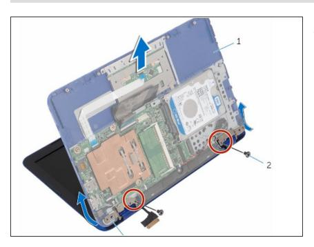
Align the screw holes on the display hinges with the screw holes on the palm rest and keyboard assembly.
