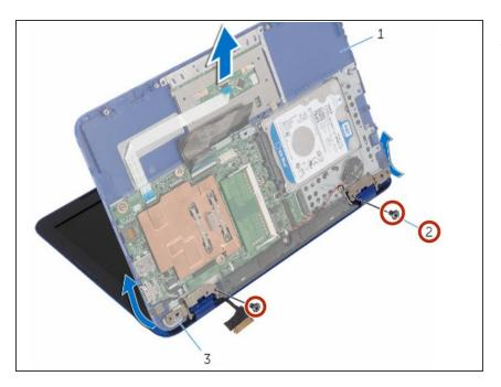
Remove the screws that secure the display assembly to the palm rest and keyboard assembly.
