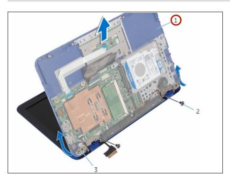
Slide and lift the palm rest and keyboard assembly off the display assembly.
