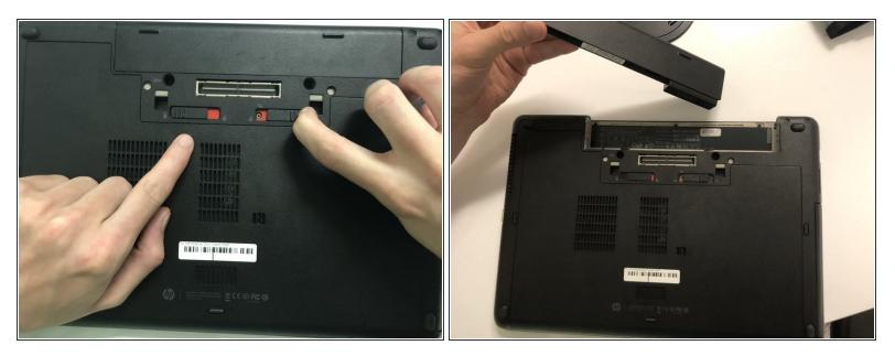
Pull on both slots outwards as shown in the images to unlock the battery. The battery will not come
