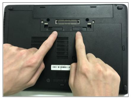
• Locate the two slots on the bottom of the laptop to unlock the battery.
