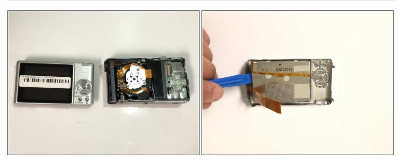
• Carefully use the opening tool to remove the LCD Screen from the glass frame.
