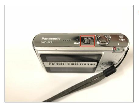
Make sure the power is off by making sure the switch is to the right. The power switch can be found on the top side of the camera.
