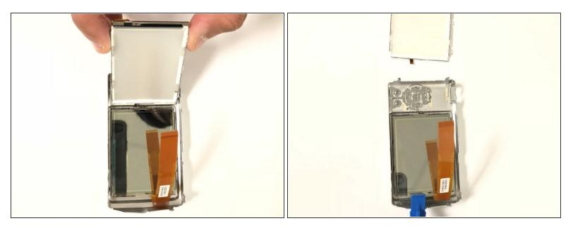
• Carefully use the opening tool to seperate the screen from the frame.
