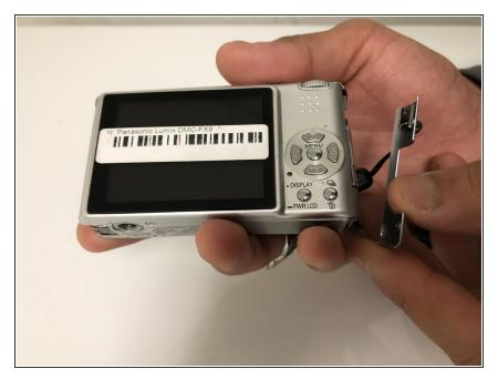
• Use the Philips #00 Screwdriver to remove the two screws on the right cover of the camera.
