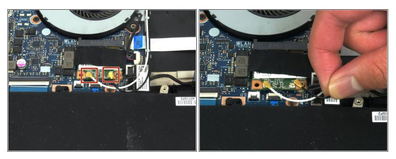
• Disconnect the white and black wires attached to the Wi-Fi chip.
