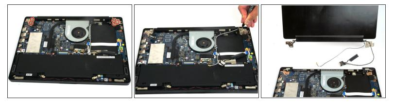
Use the JIS #0 screwdriver to remove the five 5.0 mm screws connecting the display to the rest of the laptop.
