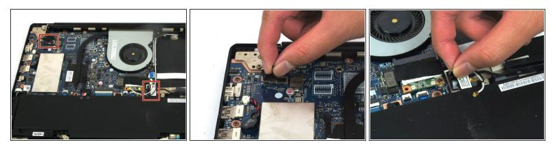
Remove the two adapters connecting the display to the motherboard by pulling the black plastic straps directly upwards.
