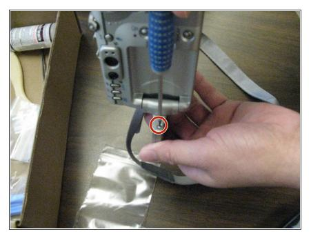
Remove both Phillips #0 screws on the opposite side of the screen, located near the hinge.
