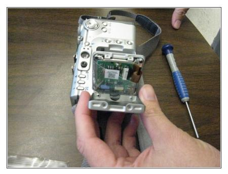
Remove the back panel of the screen, using a spudger or opening tool if necessary.
