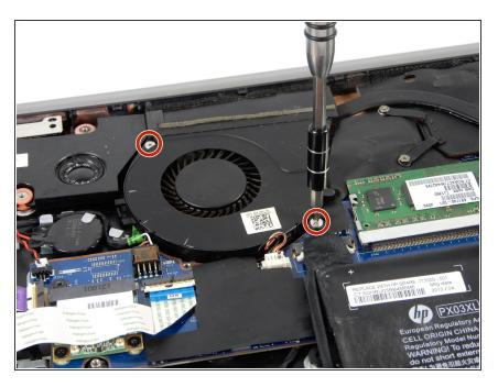
Remove two 3mm Phillips #00 screws from the fan.
