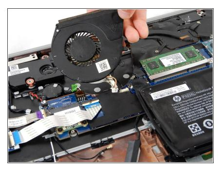
Lift the fan upwards to remove it from the computer.
