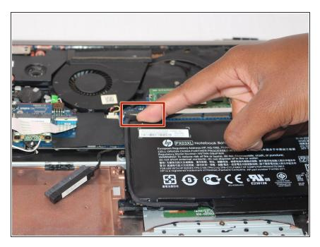
Disconnect the battery power cable from the motherboard.
