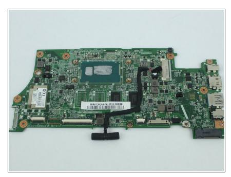
• Lift up and remove the motherboard.
