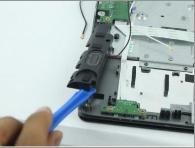
Remove the speakers located on both left and right bottom corners of the Chromebook with a plastic opening tool.
