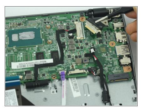
Disconnect the display cable from the motherboard.
