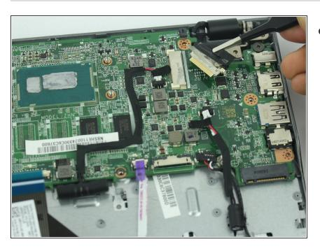
Disconnect the display cable from the motherboard.
