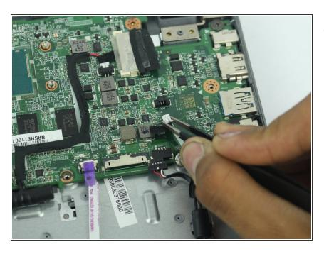
Gently pull out the wire for the 2 PIC connectors.
