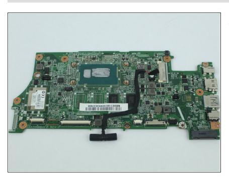
Lift up and remove the motherboard.
