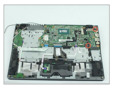
Remove the two 3.7 mm Phillips screws that hold the motherboard in place.
