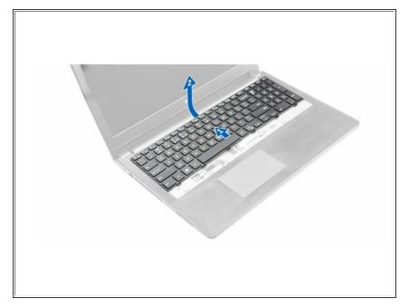
Slide and lift the keyboard to access the keyboard connector cable under the keyboard [1,2].
