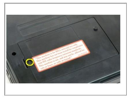
Remove the screw that secures the hard drive access panel to the base of the computer.
