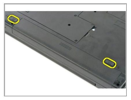
• Slide the battery lock latches into the unlocked position.
