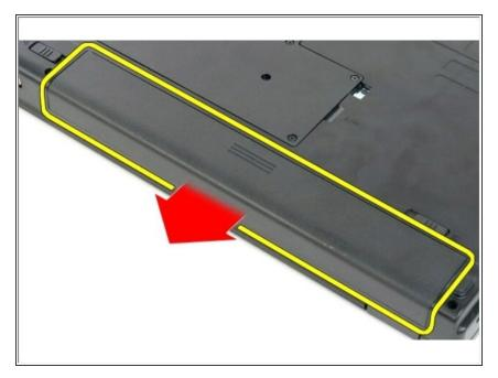
• Slide the battery toward the back of the computer to remove.
