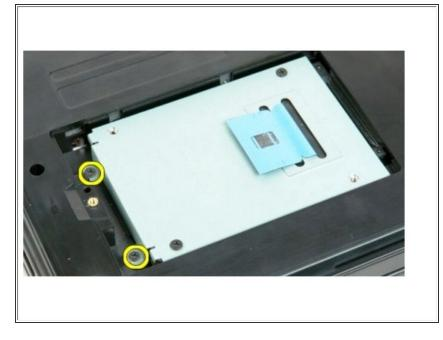
• Remove the two screws that secure the hard drive in place.
