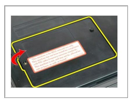
Insert a plastic scribe into the slot and lift up the access panel, then remove the panel from the computer.
