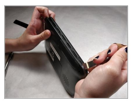
Use the spudger to remove the back cover. Insert the spudger between the back and front cover. Once inserted, you will need to move it around the perimeter to release the snaps holding it together.
