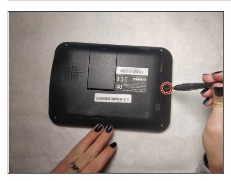
Remove the 5.0mm screw using the Phillips #0 head screwdriver.
