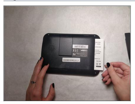
Slide the battery out by pulling on one of two plastics tabs.
