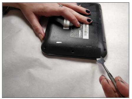
• Insert metal spudger as shown in the picture. Move spudger along to the other side until both snaps come loose.
