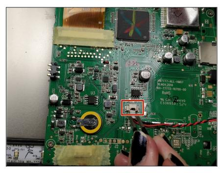
Once back cover is removed, the speaker wire will need to be removed. Use <u>tweezers</u> to remove wire.
