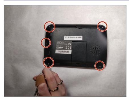
Remove the remaining five 6.0 mm Phillips #0 screws.
