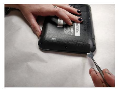
Insert metal spudger as shown in the picture. Move spudger along to the other side until both snaps come loose.
