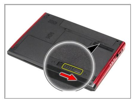
Slide the battery release latch to the unlock position.
