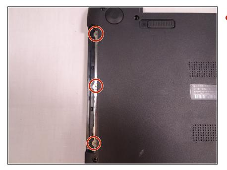
Remove the three 2mm Phillips #00 screws found underneath the disk drive.
