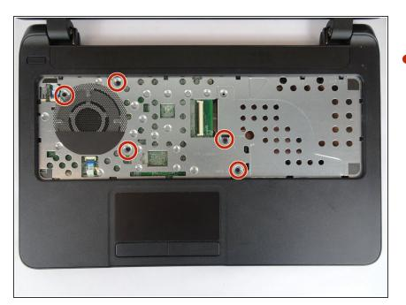
Remove the five 7mm Phillips #1 screws found underneath the keyboard.
