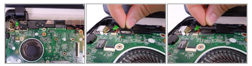
• Remove the display connection wire. Lift the connection straight up from the motherboard.
