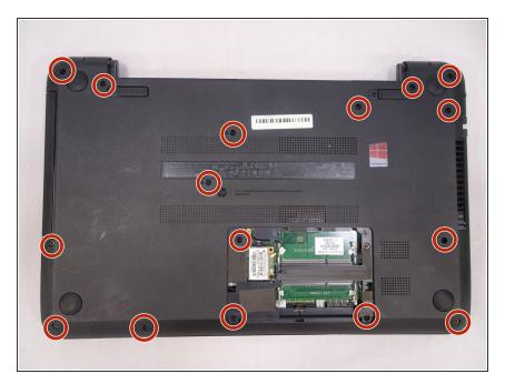
Remove the sixteen 7mm Phillips #1 screws from the bottom panel.
