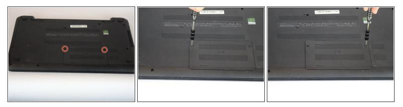
• Remove the two Phillips #1 screws from the RAM panel.
