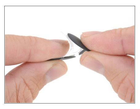
Peel a replacement foot from the plastic backing.
