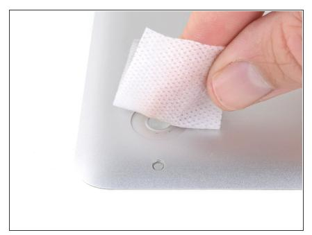
Wipe the foot pad with an alcohol prep pad to remove any residue left by the cleaner.
