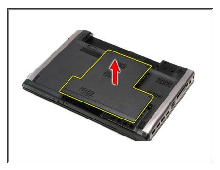
Lift up the base cover and remove it from the computer.
