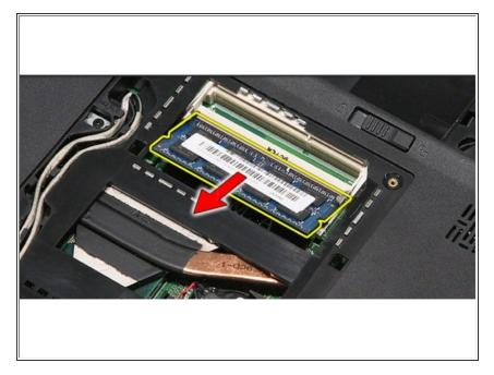
Remove the memory module from its connector on the system board.
