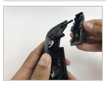
Remove the plastic trigger from the joystick.
