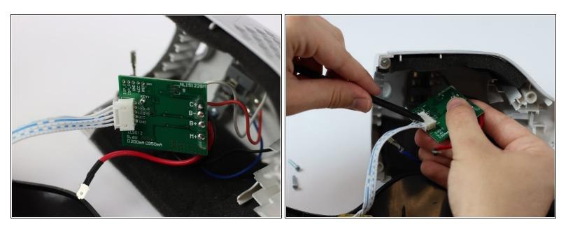
• Pry upwards on the retaining clip with black plastic spudger and pull to remove the 5 pin connector.
