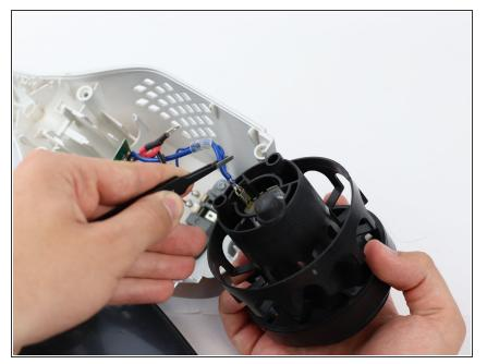
• Remove motor and impeller housing to gain access to power button.
