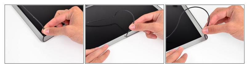
Continue pulling the display gasket off the display assembly across the top edge.
