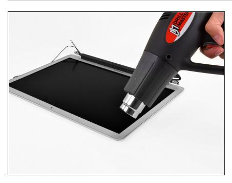
Use a heat gun to soften the adhesive under the bezel along the left and top left edges of the display.
