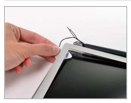
Use a guitar pick to gently lift the bottom right corner of the bezel.
