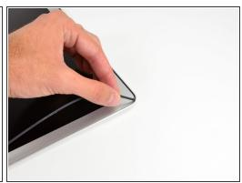
Starting with the freed corner, pull the rubber gasket off the right side of the display assembly.
