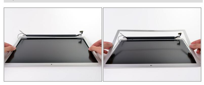
Slowly lift the bottom edge of the bezel and gently rotate it out of the display.
