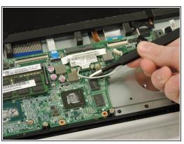
Remove the black and white wires that attach the fan to the network adapter.
