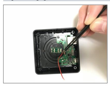
Use the <u>tweezers</u> to remove the red wire attached to the motherboard.
