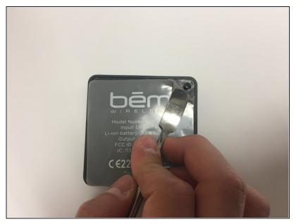
Use the metal spudger to peel back the rubber from the bottom of the auxiliary charging base to reveal the screw.
