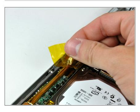
Remove the strip of tape covering the speaker cables.
