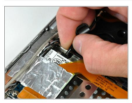
Disconnect the RJ-11 cable from the modem.
