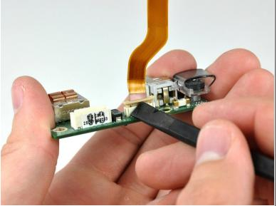
• Use the flat end of a spudger to separate the ZIF cable lock from its socket.
