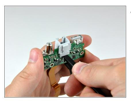
Use the flat end of a spudger to continue removing the RJ-11 board away from the DC-In board.
