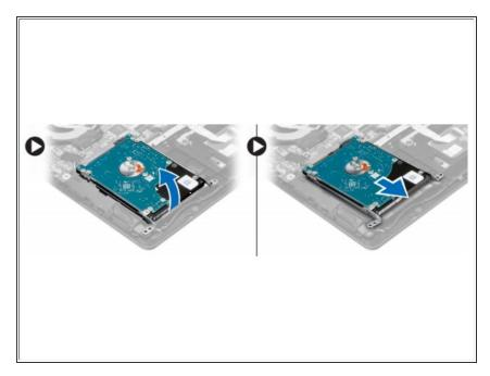
Lift the hard drive assembly in an upward direction to release it from its compartment on the computer.
