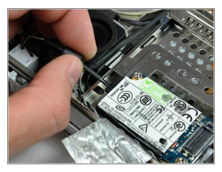
Disconnect the RJ-11 cable from the modem.
