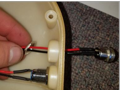
Once the cover is completely detached unscrew the nut on the back of the charging port and power button that is securing it in its place. To remove the charging port and power button push them through front of the cover.
