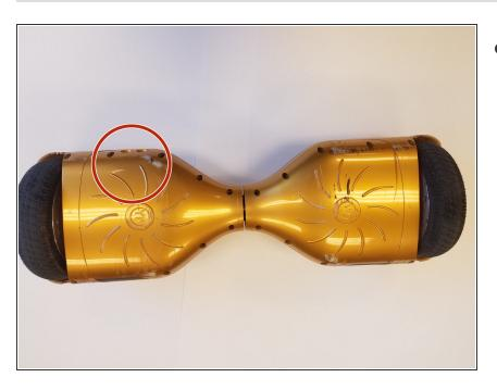
First determine which side of the board has the power button and charging port on it. Then remove the bottom cover of the board by unscrewing the 10 screws on the power button side.
