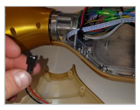
Once you remove the cover unplug the charging port, power button, and LED light to make it easier to work on.
