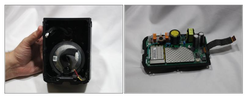
• Remove the motherboard panel from the speaker housing.
