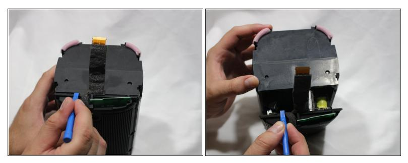
• Using a plastic opening tool, separate the motherboard from the speaker.
