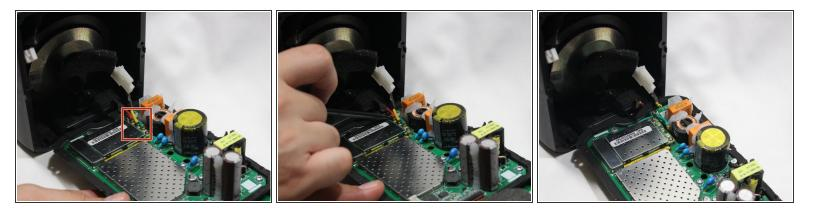
Using the pointed end of the spudger, disconnect the red, green, and yellow cables connecting the WiFi transmitter/receiver.
