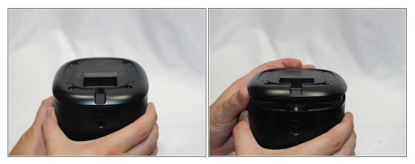
Remove the bottom cover by squeezing the protective cover slightly while pushing up with your fingers.
