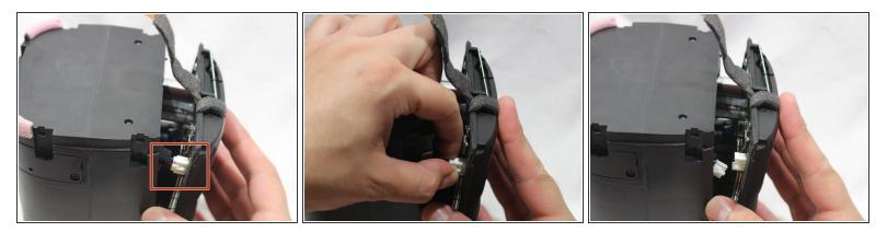
• Using your thumb, disconnect the speaker cable from the motherboard.
