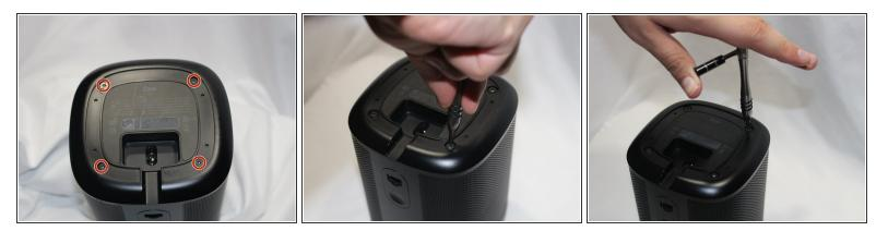
• Remove the four 10mm Torx T10 screws from the bottom of the speaker.
