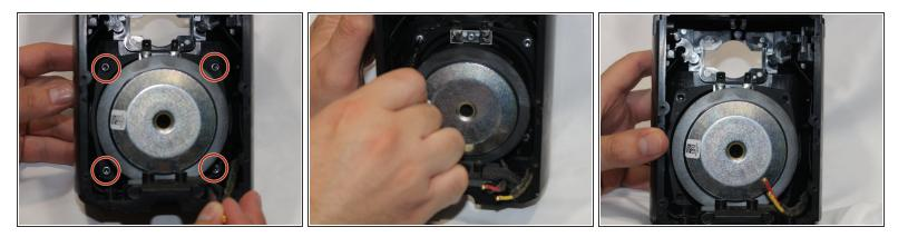
• Remove the four 10mm Torx T10 screws from the woofer.
