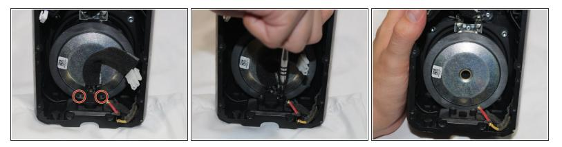
(i) The woofer is highly magnetic, making removal of the metal screws sometimes difficult.
