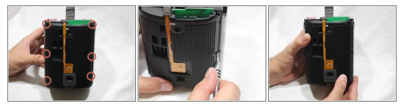
• Remove the six 9mm Torx T8 screws from the motherboard panel.
