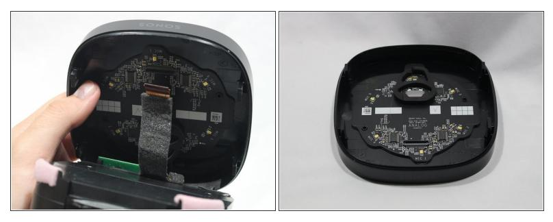
• Pull the control panel away from the speaker to separate.
