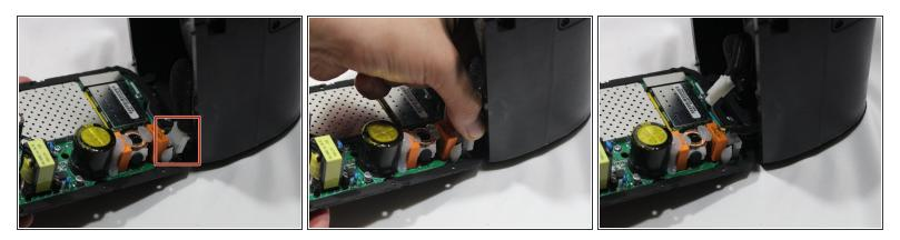
Disconnect the power adapter plug from the motherboard using your thumb.
