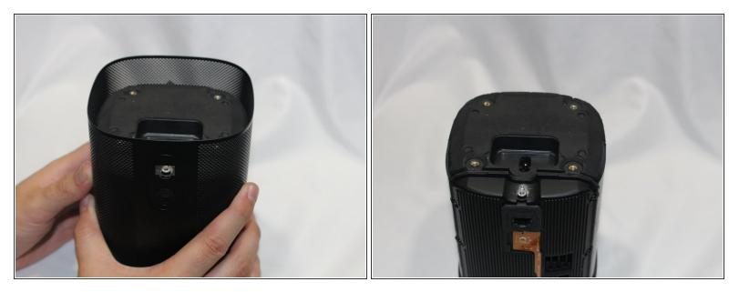
• Slide the protective cover upwards to remove.
