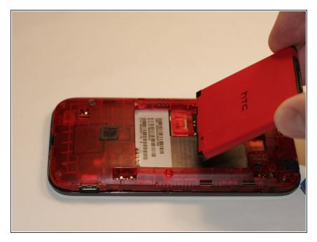
Remove the red battery to replace.
