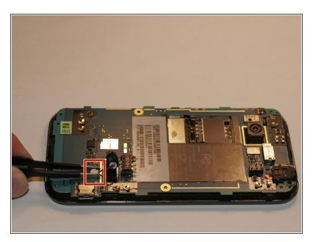
Carefully disconnect the cable attached at the motherboard.
