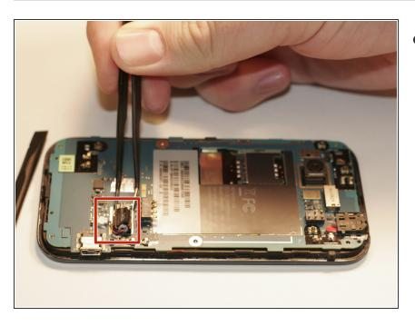
Insert the replacement's cable into the same spot on the logic board! Then just set it back into the slot on the logic board and you are done!
