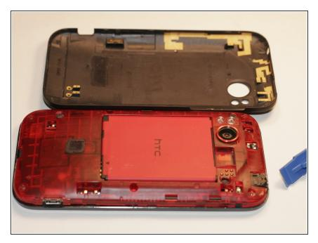
Use a plastic opening tool or your fingers to get into the groove between the cover and case.
