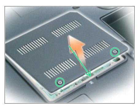
Replace the memory cover and tighten the captive screws.
