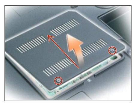
Loosen the two captive screws from the memory module cover, and remove the cover.
