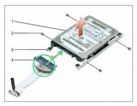
Connect the data cable to the new hard drive.
