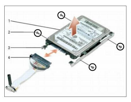
Remove the four M3 x 3-mm screws that attach the hard drive to the hard drive bracket.
