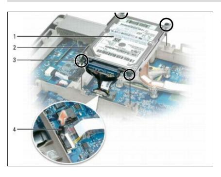
Loosen the four captive screws on each corner of the hard drive bracket.
