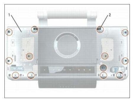
Unscrew the six M2.5 x 5-mm screws on the left side (#1) of the top cover, then unscrew the seven M2.5 x 5-mm screws on the right side (#2) of the top cover.
