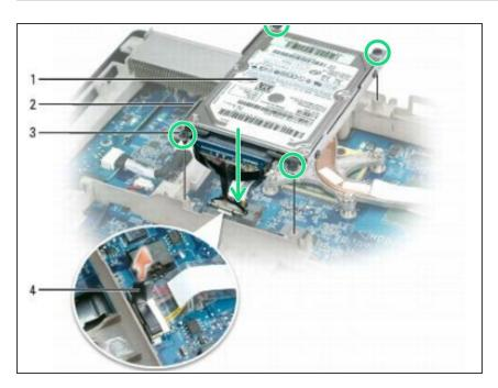
Align the captive screws in each corner of the hard drive with the holes in the frame and tighten the screws.
