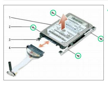
Attach the new hard drive to the brackets using four M3 x 3-mm screws.
