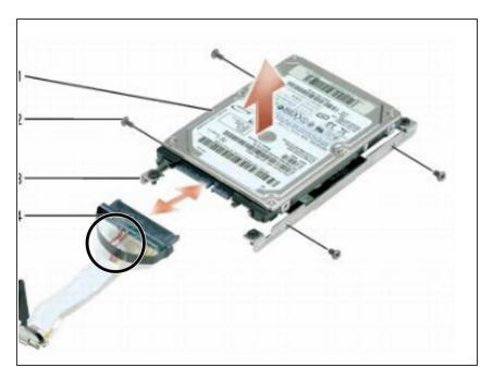
Pull the strap on the hard drive cable to remove the data cable from the hard drive. Reserve this cable for use with the new hard drive.
