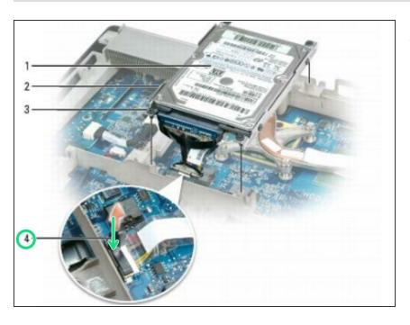
Connect the hard drive cable to the appropriate connector on the system board
