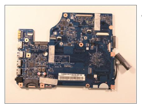
The motherboard can be replaced once disconnected from the CPU cooling fan.
